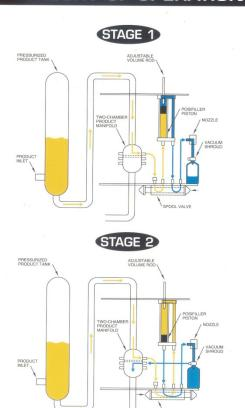
It is important to note that the **Posifiller®** is an enclosed system. No air is allowed into the system from the surge tank, through the **Posifiller®** premeasuring cylinder or through the fill nozzles.
