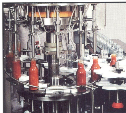
LAUBHUNT machines are designed to handle particles as large as 5/8" x 5/8" and high viscosity products like grease or peanut butter.
